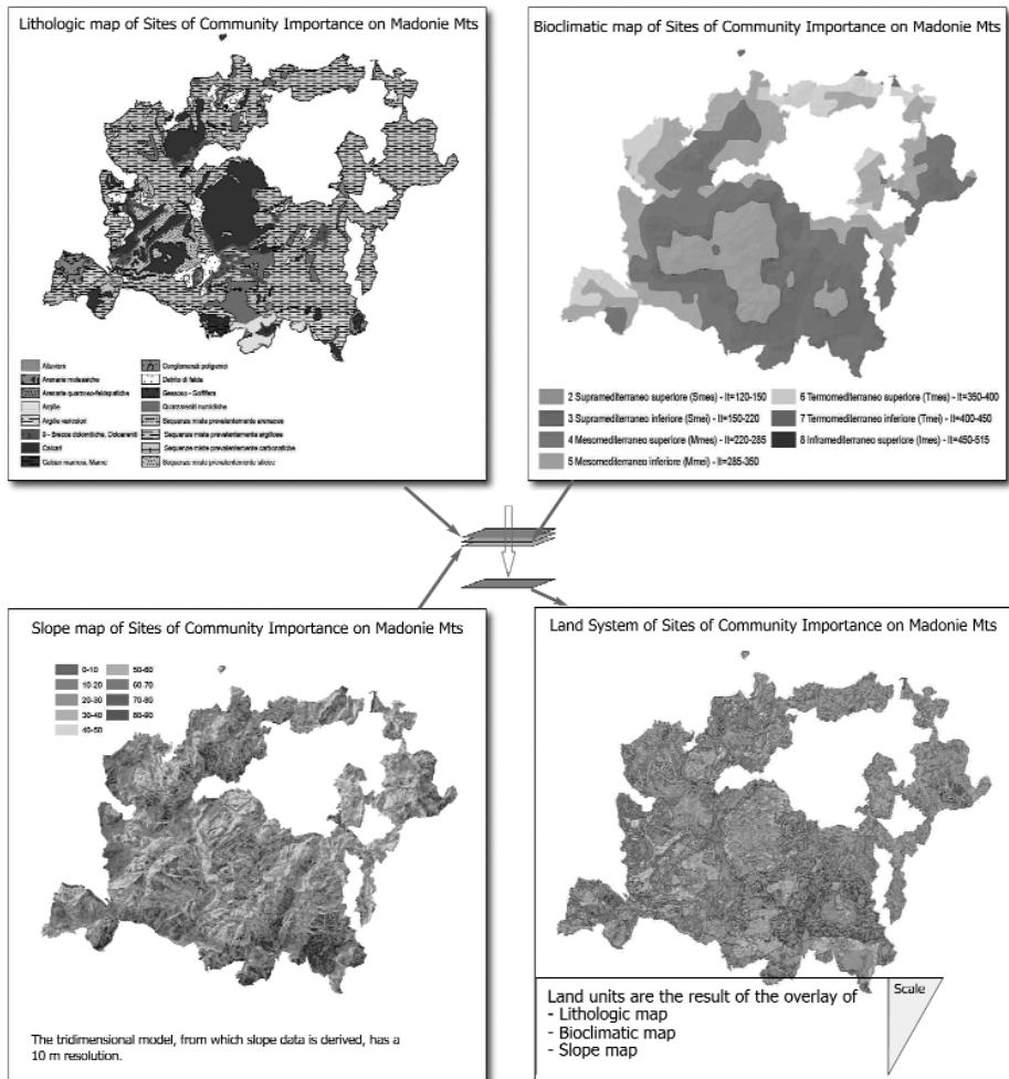
Fig. 1. Procedure illustrating the land classification. Macro-climate not represented because homogeneous on the whole area.
